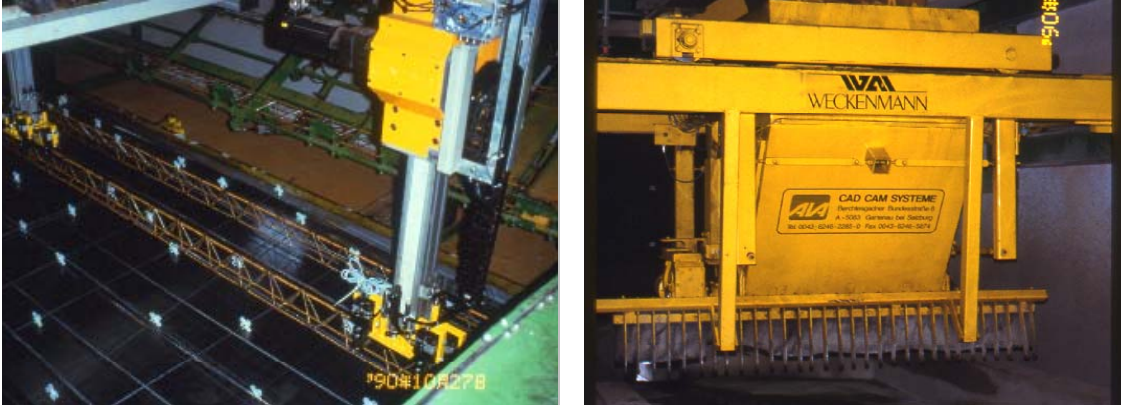
Figure 1*: Flexible CAD/CAM gantry type production unit for PC floor, wall and roof elements using two robotic end-effectors for reinforcement positioning: Figure 2*: Robotic concrete distributor
