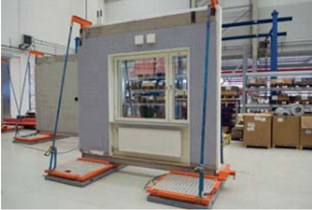
Figure 19: Concrete panel logistics in NCC factory [4].
