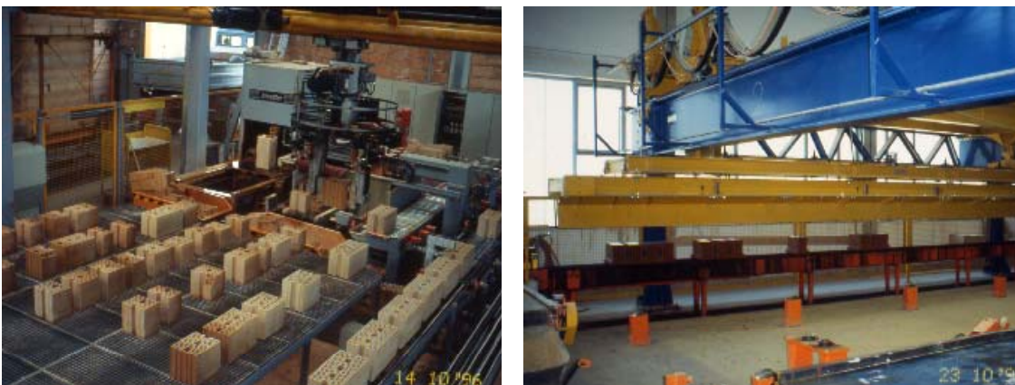
Figure 3*: Robotic cutting and sequencing of bricks Figure 4*: Robotic spacing and positioning of bricks for customized masonry wall prefabrication
