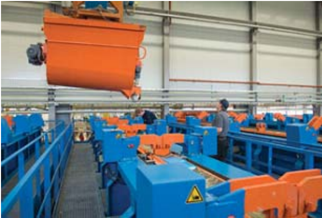
Figure 18: Concrete distribution at NCC factory(4)
