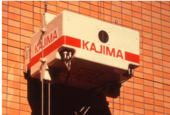
Figure 13*: Construction material distribution robot Figure 14*: Façade diagnostics robot
