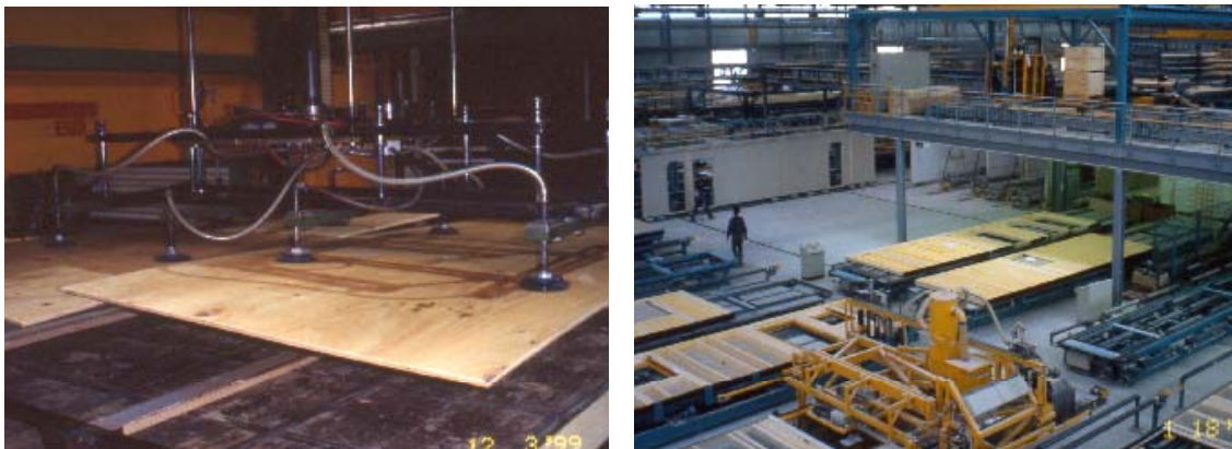
Figure 5*: Robotic vacuum gripper for customized wooden panel production Figure 6*: overview of a factory with robotic nailing and gluing bridges for wooden panel production.
