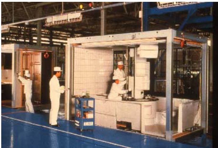
Figure 7*: Quality End Control of a box unit with bathroom from a flexible manufacturing system Figure 8*: Onsite assembly of a box unit house
