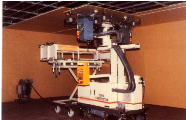
Figure 11*: Mobile ceiling drilling robot, Figure 12*: An interior finishing robot for mounting of suspended ceilings
