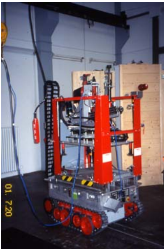
Figure 11*: Mobile ceiling drilling robot, Figure 12*: An interior finishing robot for mounting of suspended ceilings
